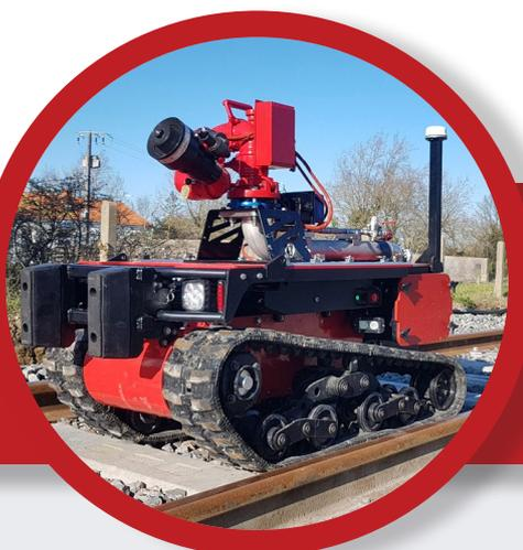
*TEC800 can perform various tasks: Fire-fighting, casualty evacuation, heavy load transportation, taking measurements (video shooting, thermography, gas, ...), ventilation, etc.*
